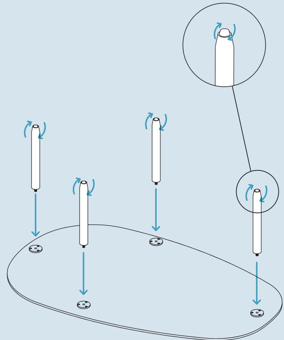
\*Legs have pre-attached adjustable levelers. Ensure unit is level prior to first use.
